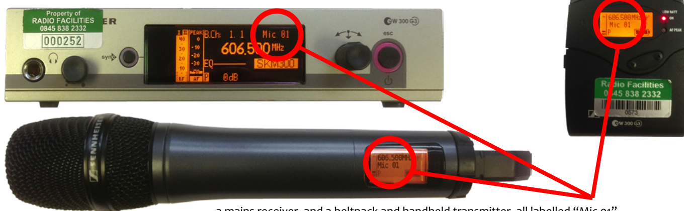
a mains receiver, and a belt-pack and handheld transmitter, all labelled “Mic 01” (note: you can only have one transmitter matched with each receiver)
